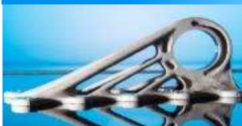
Cabin bracket "printed" from titanium powder
